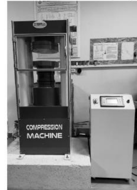
Fig. 4.1. TMC-3224 automatic compression testing machine
