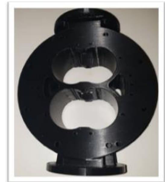
Fig.19. Hydraulic pump body printed by FDM technology
