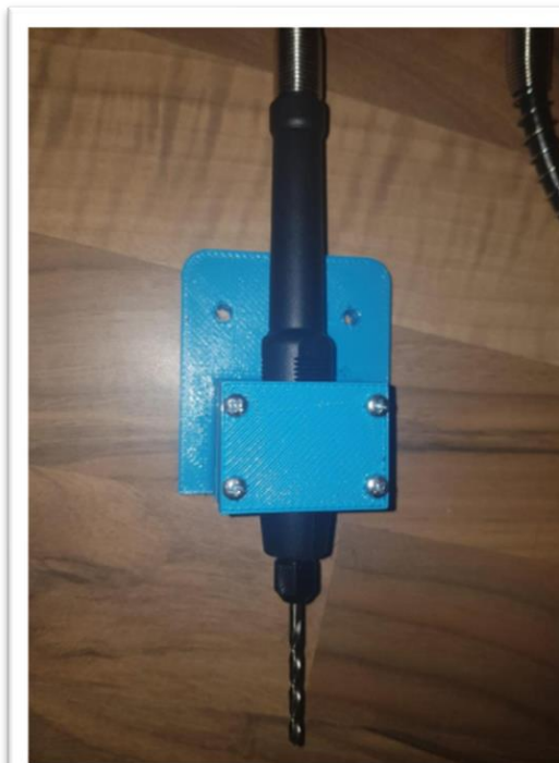
CNC head of 3D hybrid printer
