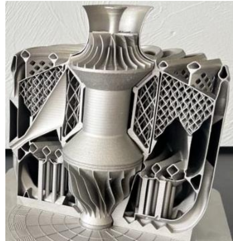
Pre-assembled micro-turbojet engine of Inconel 718 manufactured by SLM
