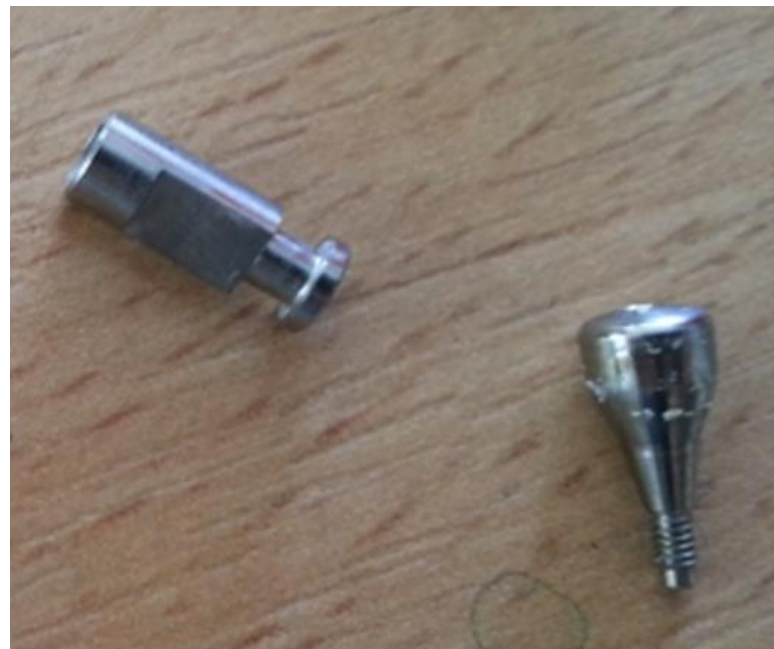
Analogue dental implants manufactured via DMLS
