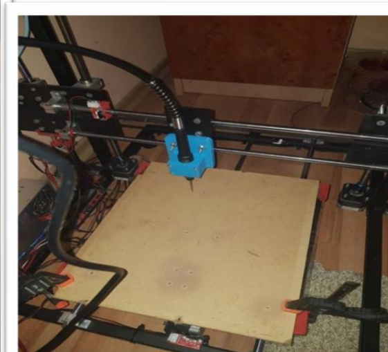
CNC drilling on the 3D hybrid printer.
