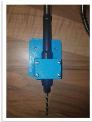
Fig.21. CNC head of 3D hybrid printer
