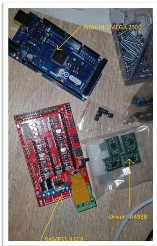
Fig.9. Arduino MEGA 2560 board
