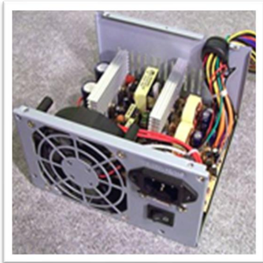
Fig. 11. Power supply PC PSU 12V 14.6
