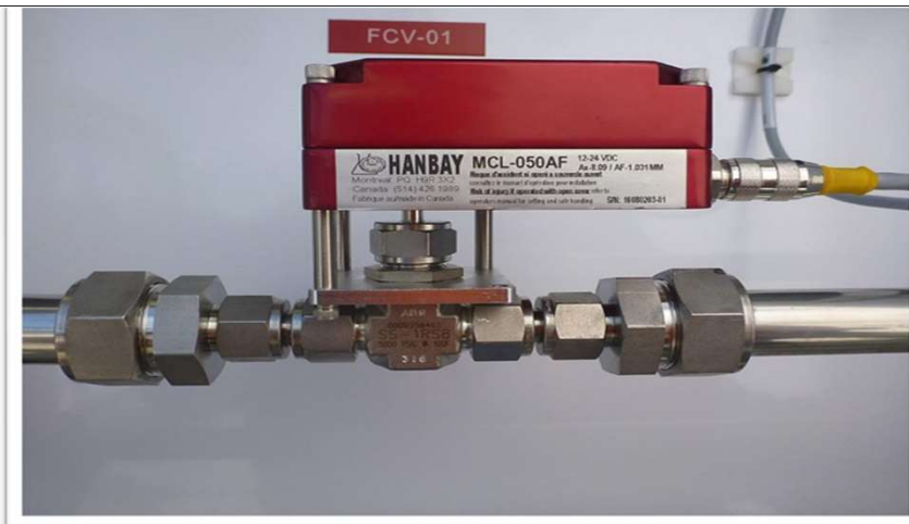
Fig.5. Electric valve actuator controlling a 1/2 needle valve [6]
