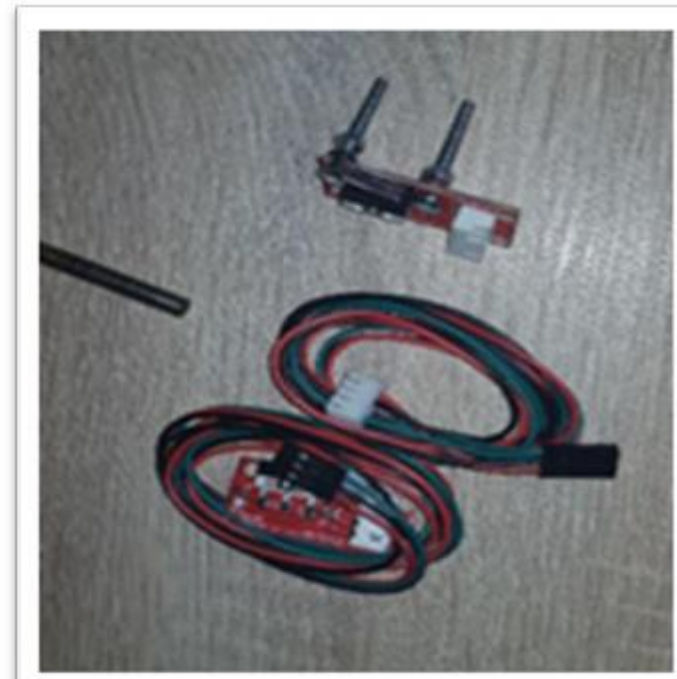
Fig. 12. Endstop with mechanical feeler
