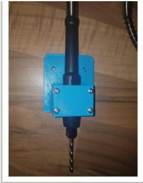
Fig.21. CNC head of 3D hybrid printer
