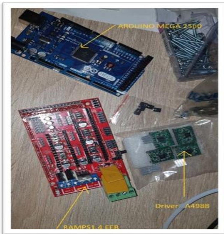
Fig.9. Arduino MEGA 2560 board
