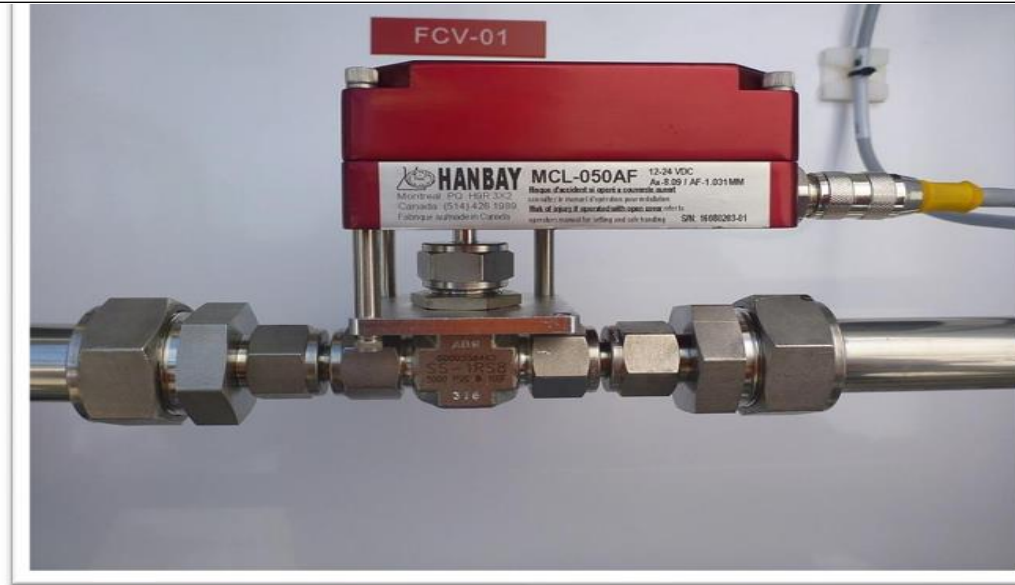
Fig.5. Electric valve actuator controlling a 1/2 needle valve [6]
