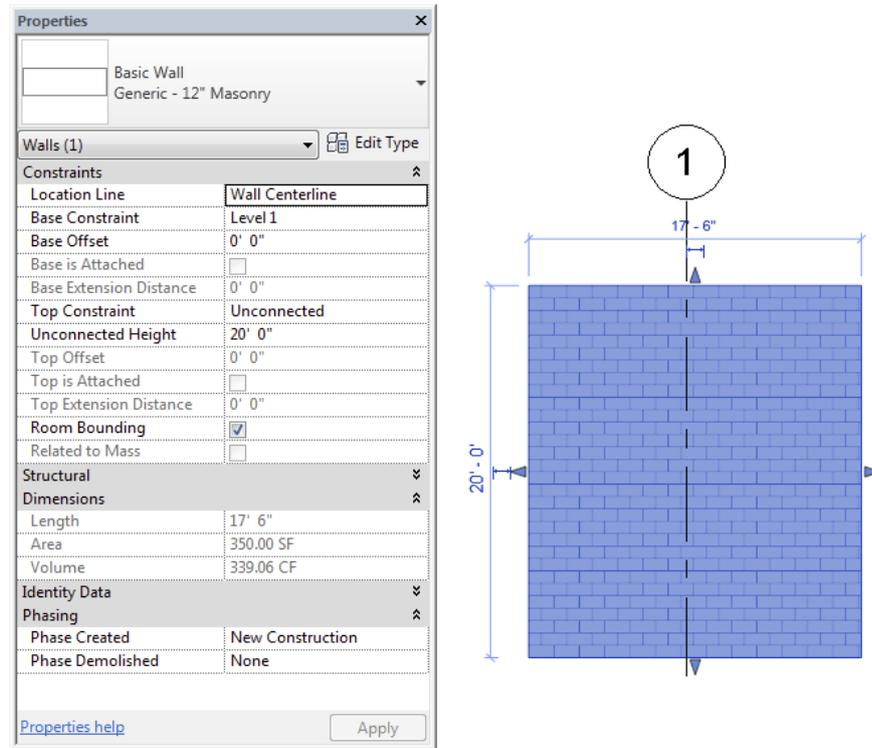
Fig. 8. Parameters of the wall instance
