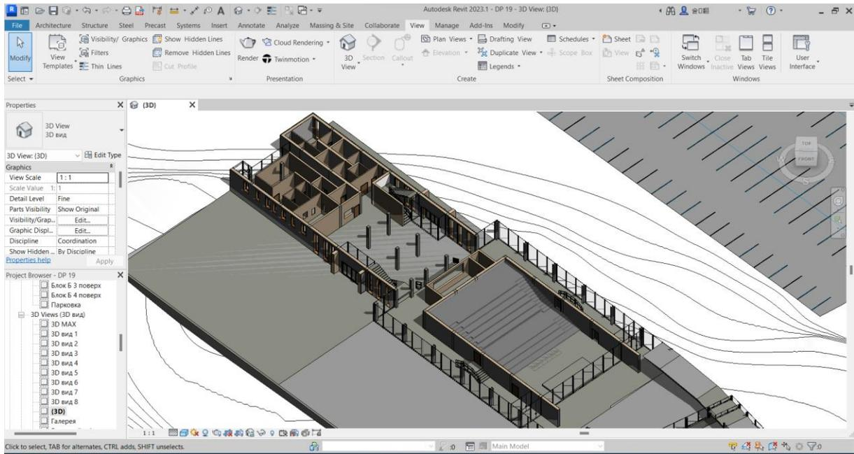
Fig. 22. 3D section in Revit [13].
