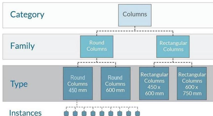
Fig. 10. The "column" element in the Revit structure
