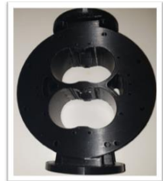
Fig.19. Hydraulic pump body printed by FDM technology
