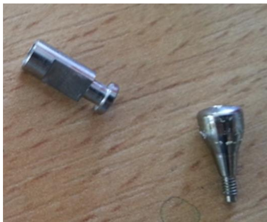
Fig.15. Analogue dental implants manufactured via DMLS
