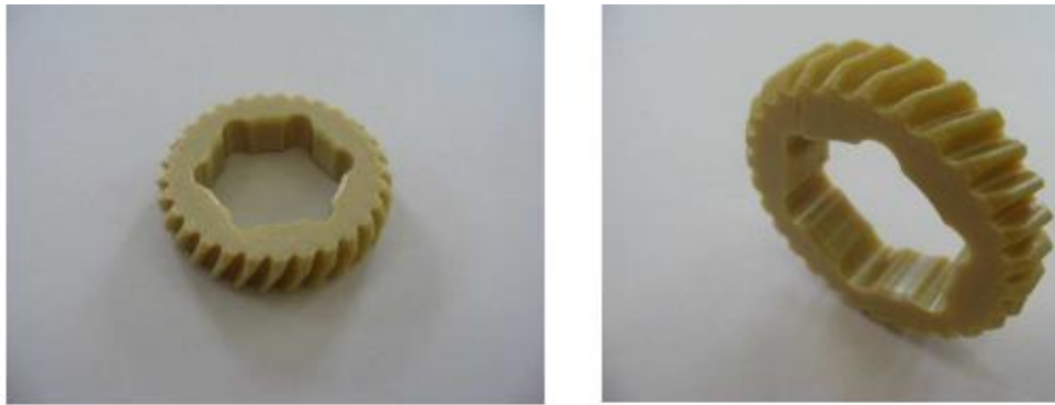
Figure 4.5. New gear wheel made from ULTEM 9085 [65]
