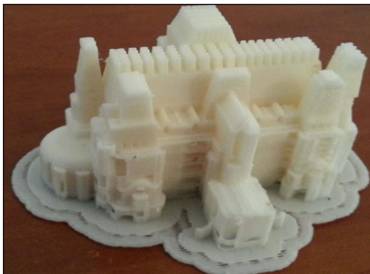
Fig.7. Resins used in architectural domain (Kretzulescu Palace) manufactured by SLA
