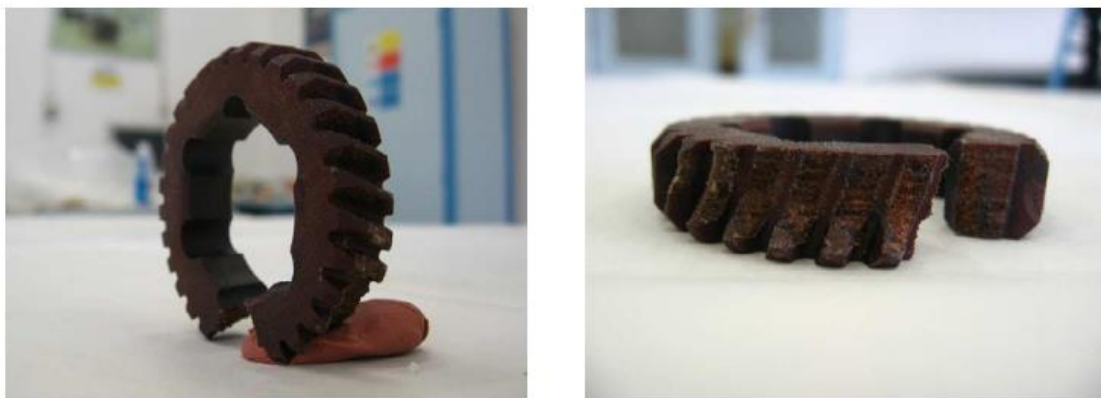
Figure 4.1. Damaged component – gear-wheel [65].
