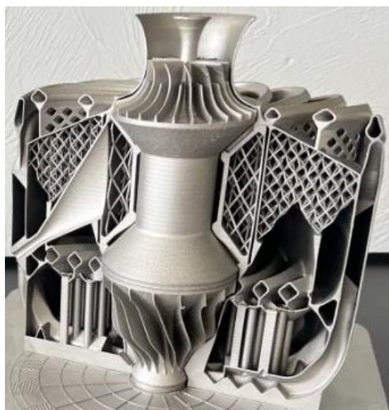
Fig.17. Pre-assembled micro-turbojet engine of Inconel 718 manufactured by SLM [122]
