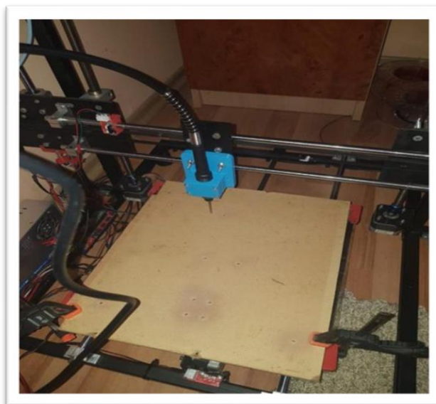
Fig.22. CNC drilling on the 3D hybrid printer
