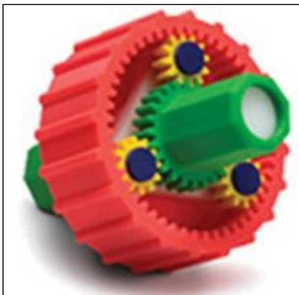
Fig.2. Assembly of parts obtained by the FDM process [20]
