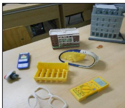
Fig.9. Parts manufactured by DLP technology
