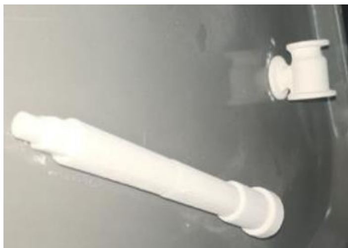
Fig.22. Industrial part manufactured by Binder Jetting using Zprint 310 Plus system
