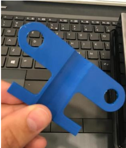
Fig.11. The cable fixing clamp printed using FDM technology, after cleaning the supports
