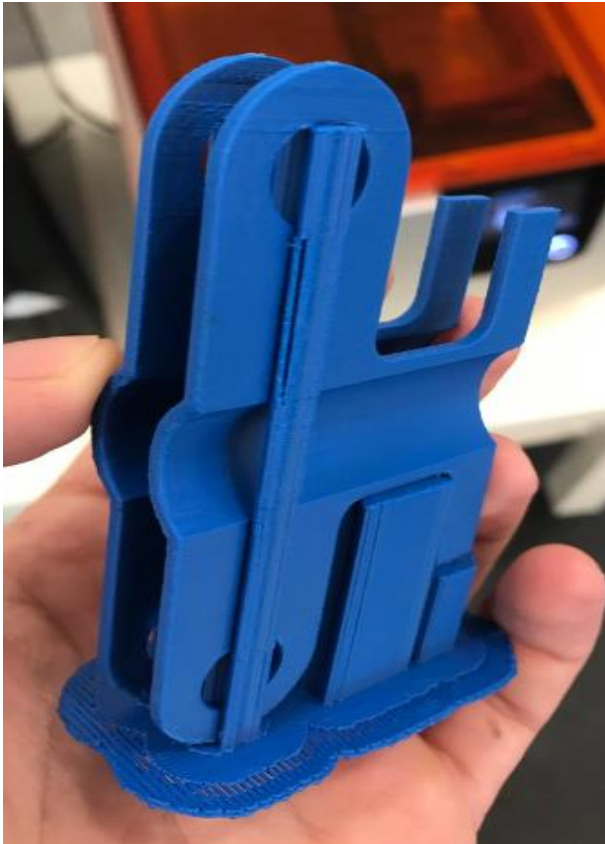
Fig.10. The cable fixing clamp printed using FDM technology, with supports
